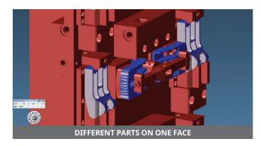
The ability to generate CNC code in single-part mode to prove set up and machining before running a fully loaded tombstone Optimization is typically dependent on grouping similar or identical operations together to minimize tool changes and rotations of the tombstone. TMS lets the programmer:
